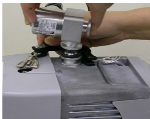
Figure 9 Mount Inlet Valve with IDP-3 Pump
